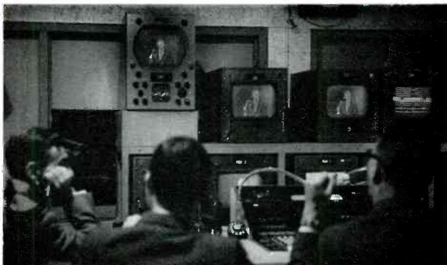
ABC-TV engineers control video portion of closed circuit telecast. Monitor shows grey scale with black level at bottom and white level at top.
